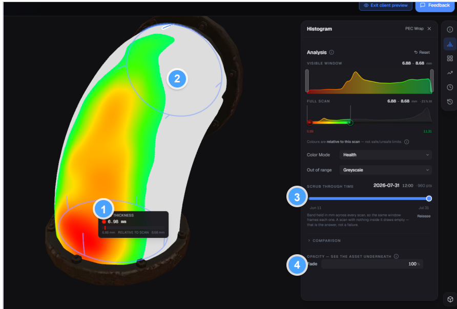
Hover tooltip and scan-history scrubbing on a PEC-wrap elbow. HELIX demonstration asset (Erosion Elbow Demo).
