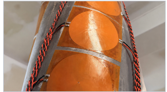
HELIX Sensor Wrap: planar spiral coils wound over the spool. Patent-pending, tileable across diameters.
