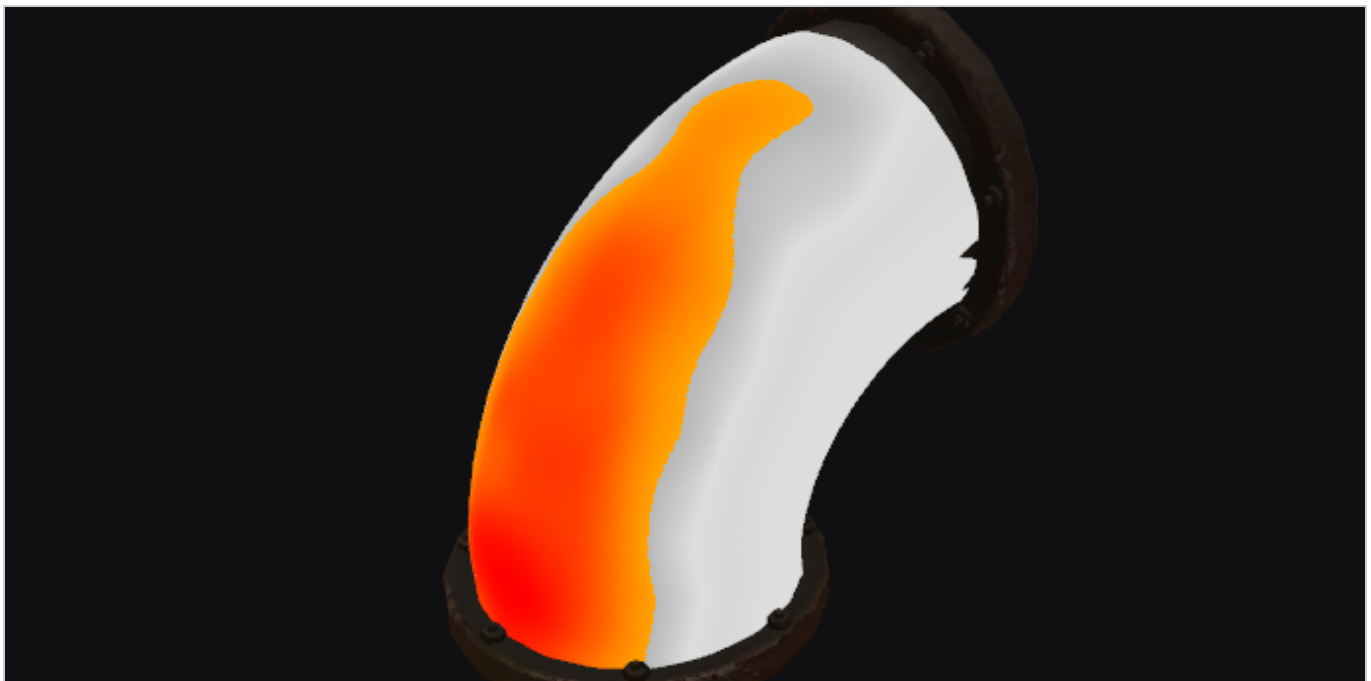
The instrumented demonstration elbow in HELIX Horizon — red marks the thinnest wall. Simulated data. Colours are relative to this scan — they mark the lowest and highest readings shown, not safe/unsafe limits.
